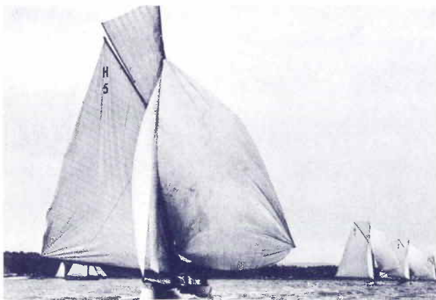
Six Metre racing in 1910. It will be seen that the rig is the conventional gaff rig with topsail. The "H" was an early class designation in England.
